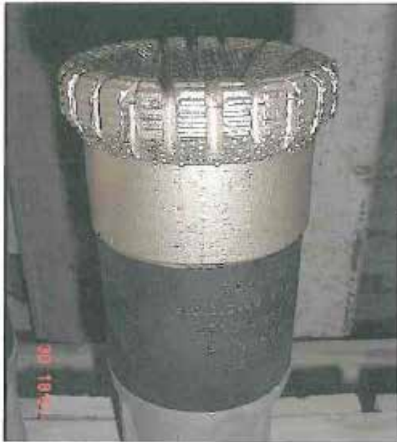
Fig. 5 Cement ramp Window mill
