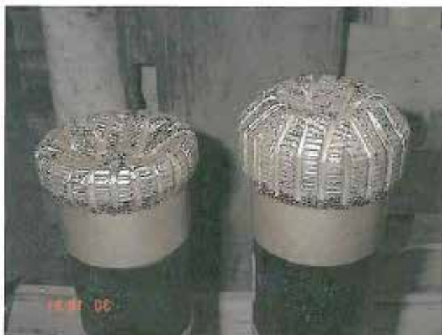
Fig. 6 Cement Ramp Mill & One trip Window mill
