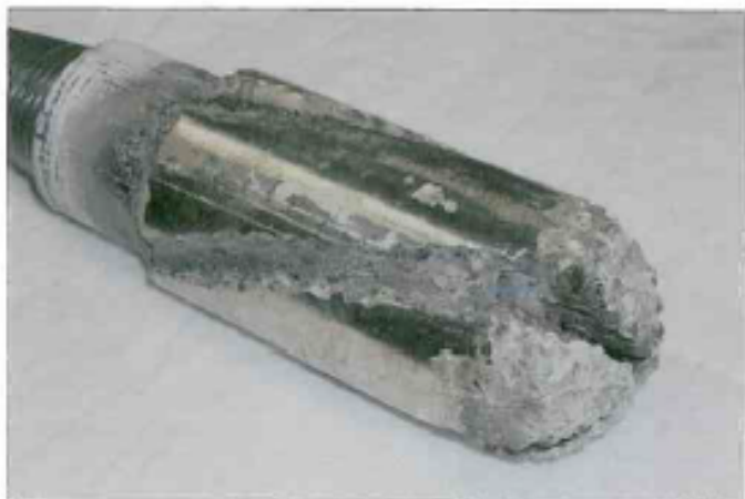
Fig. 3 Carbide Formation mill (3.625" OD)
